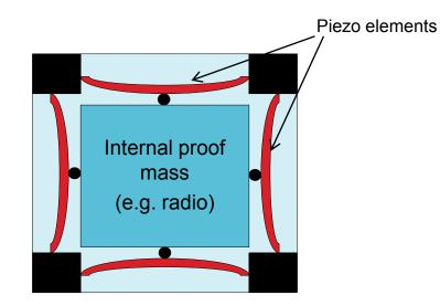
MFC-P1 type MFC-P3 type MFC-P2 type Bimorph PVDF2 PVDF1 THUNDER Initial testing in context of "leaf-spring" suspension of internal proof mass
