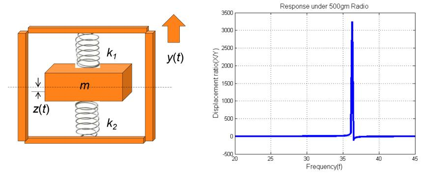
Given the compliance of the piezo elements and gait frequency, movement of soldier will not be coupled to proof mass.
