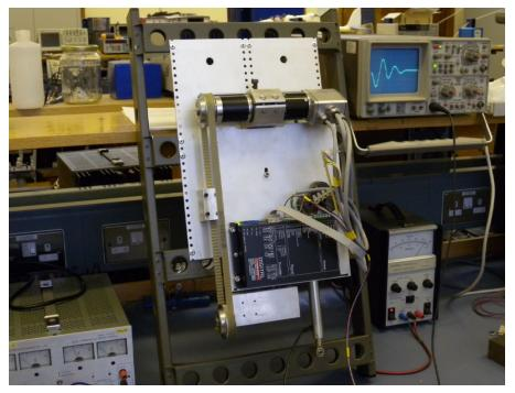
Frictional losses in mechanism investigated, allowing parasitic damping to be reduced.
